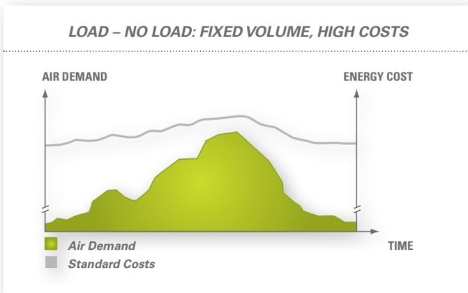
Traditional compressors working with a full load, no load control operate between two set pressure points. When maximum pressure is reached, the compressor goes off load. During periods of medium to low air demand, the no load power consumption can be excessive – wasting large amounts of energy.
