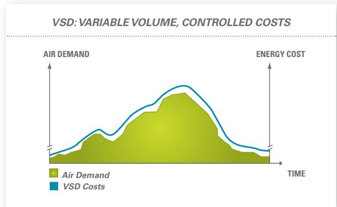
Because there is no unnecessary power generated, the GA VSD can reduce energy costs by 35% or more. Lifecycle costs (LCC) of the compressor can be reduced by an average of 22%. In general, the extra cost of a VSD compressor compared to a fixed speed one can be earned back after just one to two years.
