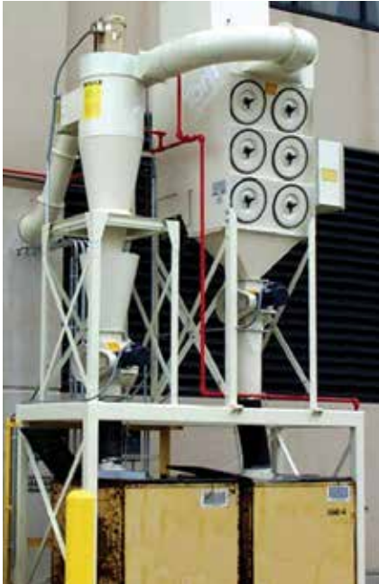
DFT/CYCLONE on Paper Processing 5,300 cfm (9,003 m 3 /h)
