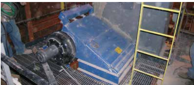
CPV - Bucket Elevator 1,200 cfm (2,038 m 3 /h)
