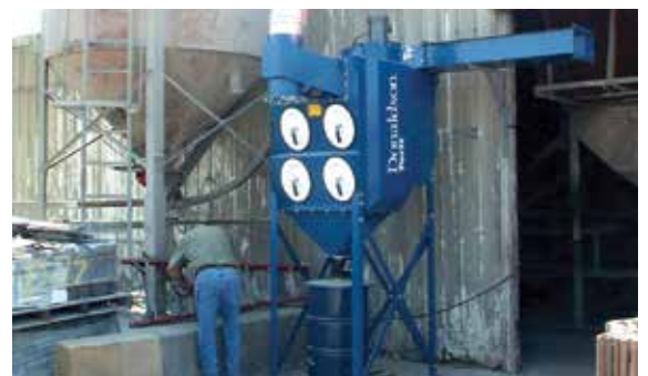
DFO - Concrete Roof Manufacturer 3,000 cfm (5,096 m 3 /h)
