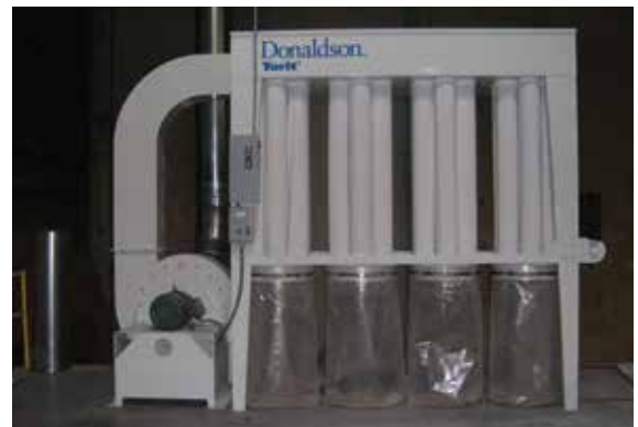
IRD - Wood Shop 5,000 cfm (8,493 m 3 /h)
