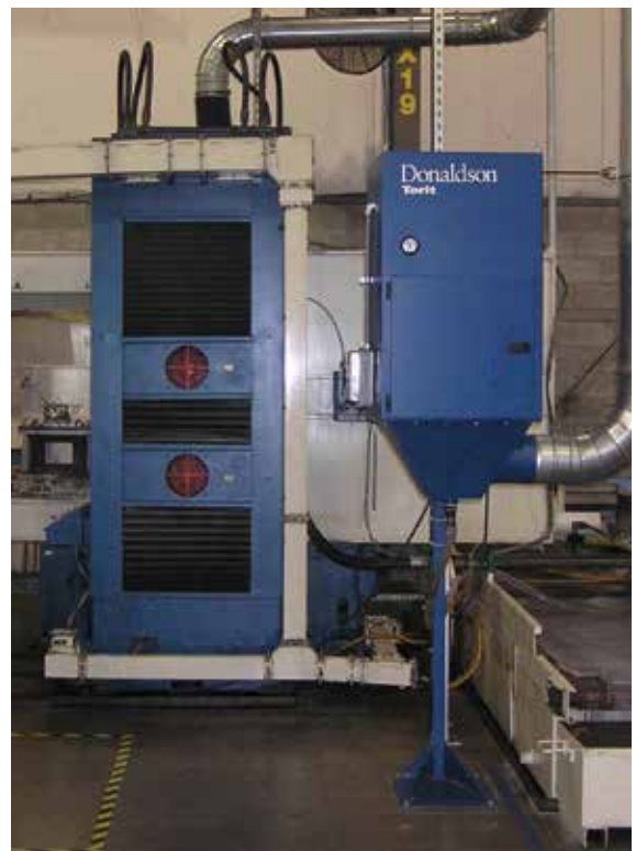
WSO - Horizontal Grinder 850 cfm (1,444 m 3 /h)
