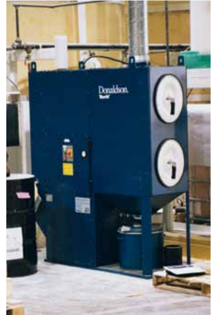
DFO on Paint & Pigment 1,200 cfm (2,038 m 3 /h)
