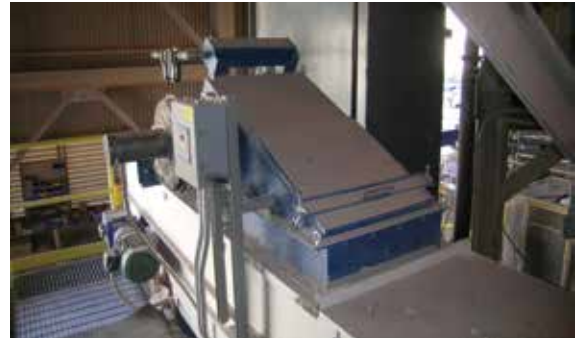
CPV - Weigh Belt Feeder 800 cfm (1,359 m 3 /h)
