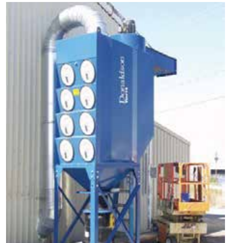
DFO on Plasma Cutting 5,000 cfm (8,493 m 3 /h)
