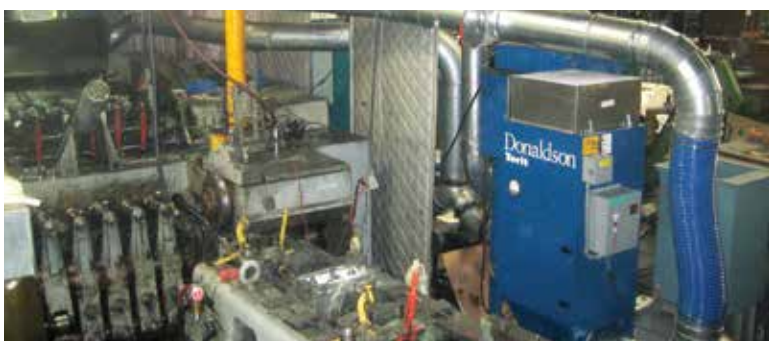
WSO on Cold Forming 1,200 cfm (2,038 m 3 /h)
