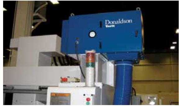
DMC on Wet Machining 390 cfm (662 m 3 /h)
