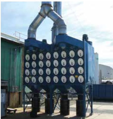
DFO on Thermal Spray 8,500 cfm (14,439 m 3 /h)
