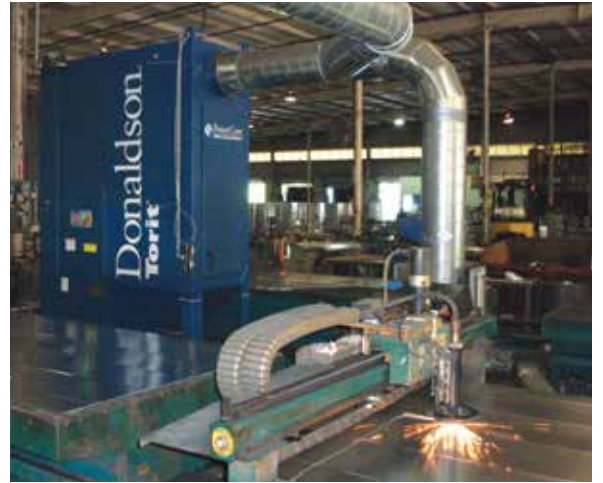
TG on Plasma Cutting 3,400 cfm (5,775 m 3 /h)
