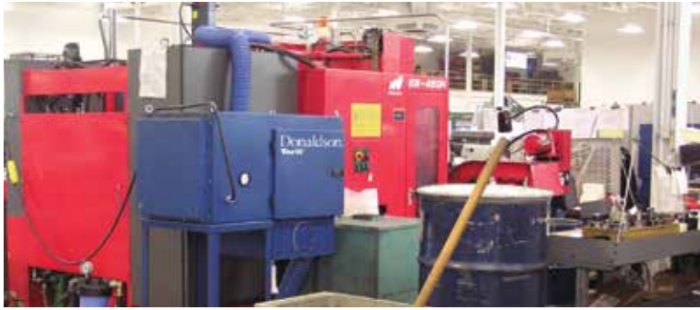
DMC on Machining 800 cfm (1,359 m 3 /h)
