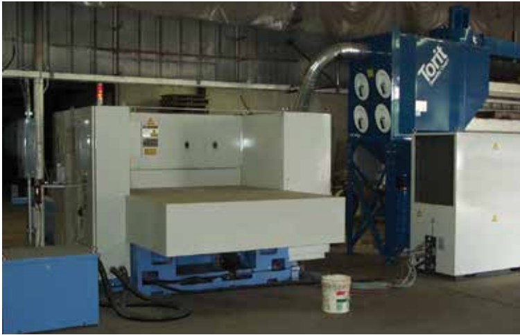
DFO on Laser Cutting 3,100 cfm (5,266 m 3 /h)
