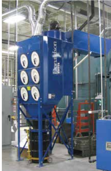
DFO on Rubber Grinding 2,500 cfm (4,247 m 3 /h)
